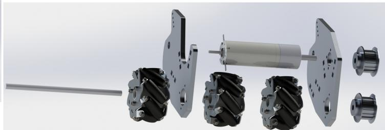
**Fig. 8.** Exploded view of the left part of the ball handling system.
