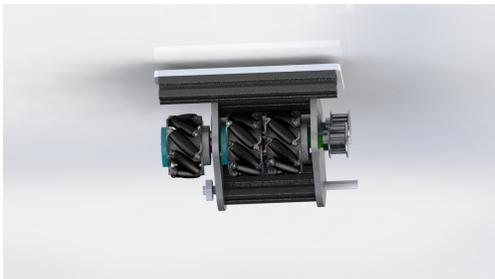
**Fig. 7.** Left part of the ball handling system composed of 3 mecanum wheels driven by a Maxon DCX26 motor.
