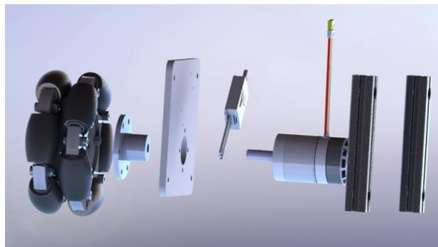
**Fig. 3.** Propulsion block including a Robotmaster M3508 motor with a C620 speed encoder
