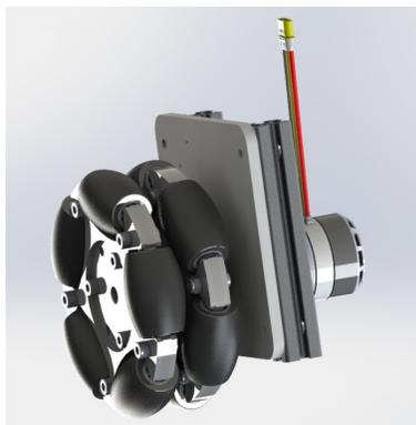
**Fig. 2.** RCT propulsion element
