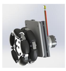
Fig. 5. RCT propulsion element
