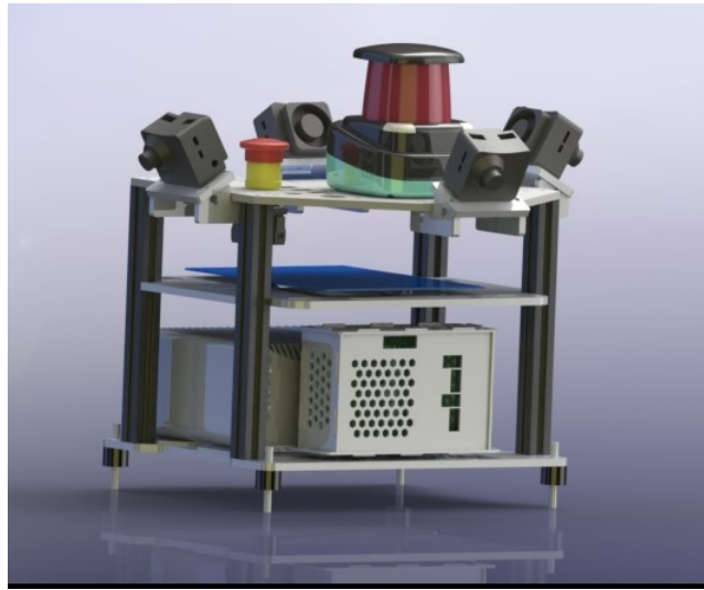
Fig. 9. Top assembly of the robot including the embedded PC and the motor controller board for driving motors and managing quadrature encoders. This assembly can be removed from the robot by removing 4 screws for transportation. A Pepperl+Fuchs R2000 lidar is present as well as four JeVois Pro smart cameras.
