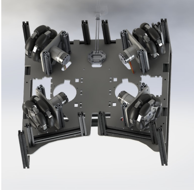
Fig. 4. RCT omnidirectional base view showing motor blocks, power distribution and control board card and bottom chassis
