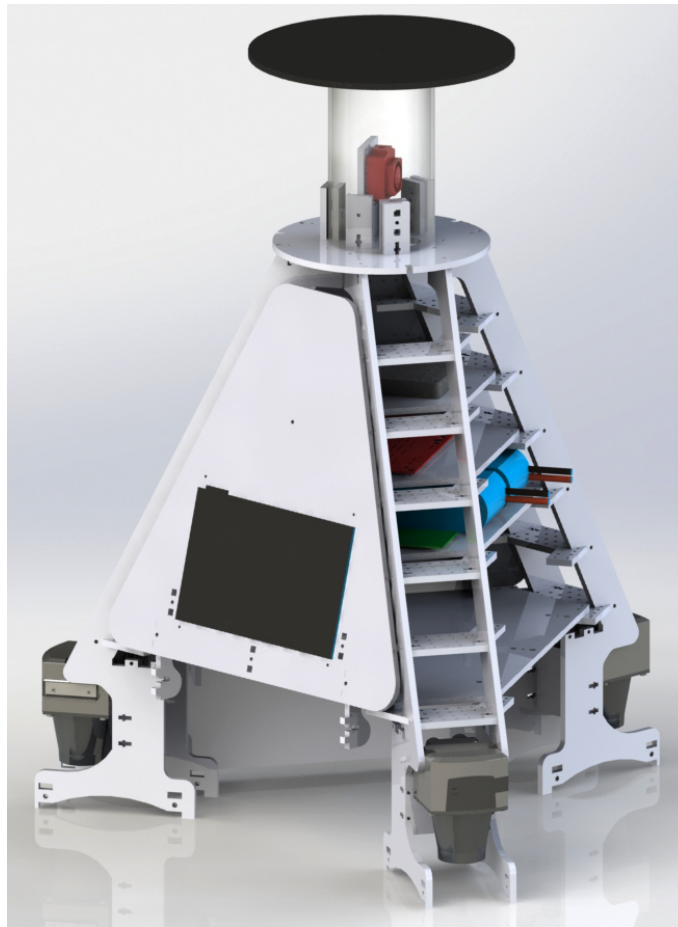
Fig. 11. Top pyramid of the robot including the embedded PC, display screen, and the peripheral board for driving motors and managing quadrature encoders. This assembly can be removed from the robot very quickly removing only 12 screws. Sick TIM361 LIDARs are in their final position on this view (only 2 LIDARs will be present in the final robot).
