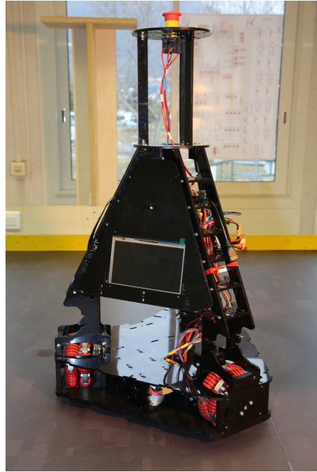
Fig. 1. Computer generated image of the 2019 robot of Robot Club Toulon Team in its latest version including a PMMA transparent tube at the top for the camera, and picture of the robot in an older version and without the ball control system.
