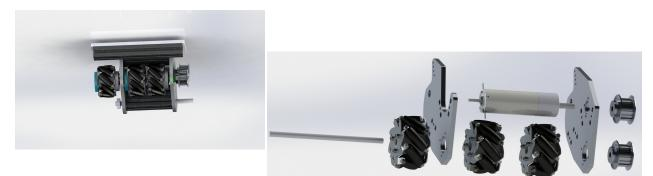
Fig. 7. Left part of the ball handling system composed of 3 mecanum wheels driven by a Maxon DCX26 motor.
