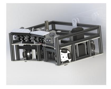
Fig. 6. RCT omnidirectional base with kicking and ball handling systems
