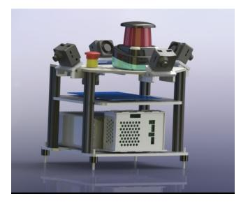
**Fig. 9.** Top assembly of the robot including the embedded PC and the motor controller board for driving motors and managing quadrature encoders. This assembly can be removed form the robot by removing 4 screws for transportation. A Pepperl+Fuchs R2000 lidar is present as well as four JeVois Pro smart cameras.
