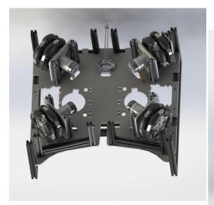
**Fig. 4.** RCT omnidirectional base view showing motor blocks, power distribution and control board card and bottom chassis
