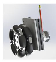
Fig. 2. RCT propulsion element
